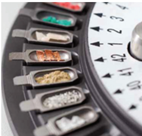
Fig. 12. The integrated microbalance (a) and autosampler (a, b) of the direct solid samples analyser through GF-AAS
