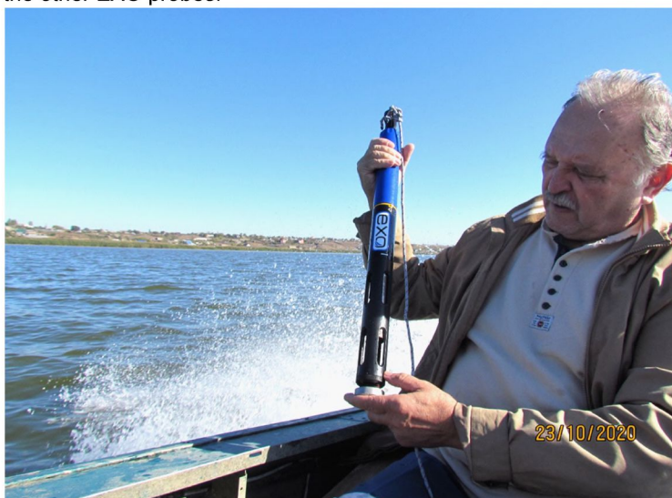
Fig. 3. Multiparameter hydrological sonde EXO1 that collects water quality data
