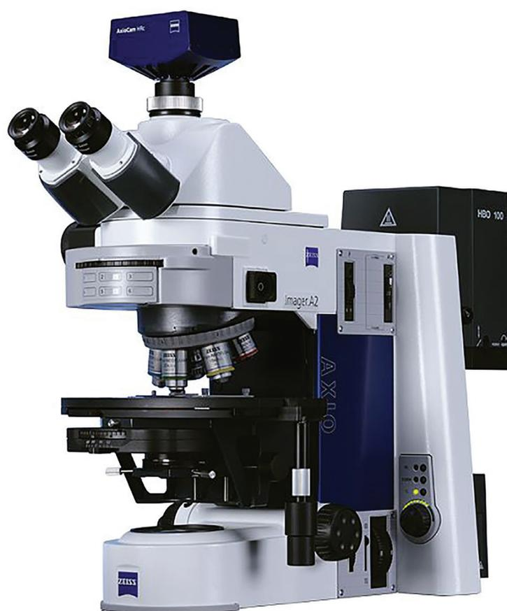
Figure 4.2. Computerized microscope Axio Imager A.2 (Zeiss)
